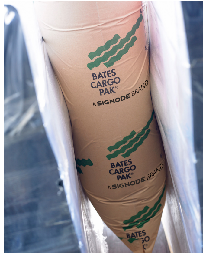
Flex airbag inflated in position
